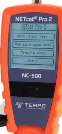
When used with the NC-510 Accessory Kit, containing seven (7) expansion remote test modules, the NETcat® Pro2 can uniquely test coax or twisted pair jacks from a central location eight (8) at a time. Using a fingertip or the built-in stylus, the screen can be used to control and display a range of tests from fault finding to TDR length measurement. The display can be set to English, Spanish, French or German language.
